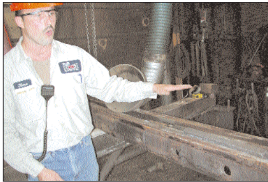
Our guide, Steve Basham shows a relay frog in which cracks and other material are cut out, and manganese is welded to the surface.
