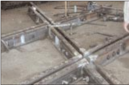
Koppers' Industrial Track Work division also manufactures crossings. Seen above is a new 132RE 61° tangent/curve two rail bolted crossing for industrial track.
